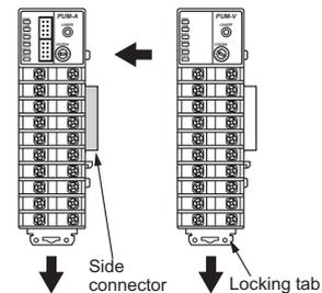
3. After mounting controllers onto DIN rail, make sure to push up all locking tabs. Controllers are fastened to DIN rail and to each other.
