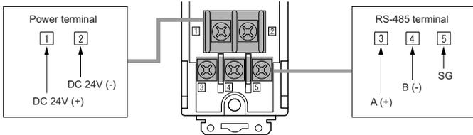
All connected controllers are connected to power supply and RS-485 via side connectors if one of controllers is directly connected to them.
