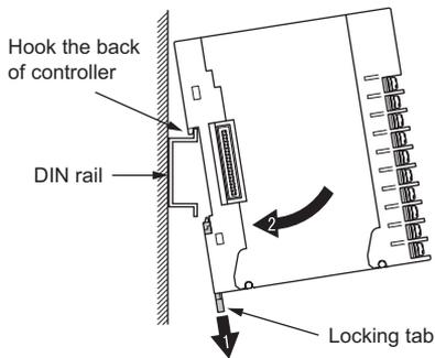
3. Push up the locking tab to fasten the controller onto DIN rail.
