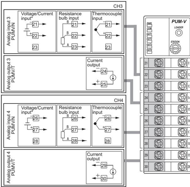
\*In case of current input, attach I/V unit which comes with the controller to the voltage input terminal.
