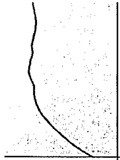
Setting too wide slow warm up and poor control
