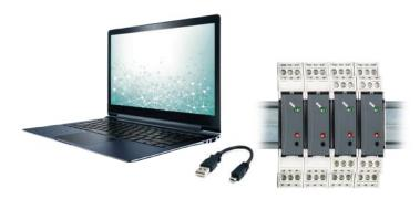
A standard Micro USB cable (our code is CCX) is required to connect COMPACT to the computer. The Windows driver for the USB connection is installed by the setup software installer.
