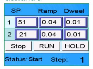
Pushing the START button on the menù is possible to open an Operator Pop Up, where is possible to Run, Hold or Stop concurrently all the program stored for each loop.
