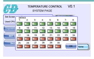
**Advanced Setting Page**: It's very easy to add or remove one zone on the software. Each loop can be enabled or disabled by pressing a push button. For each zone is possible to set a dedicated name.
