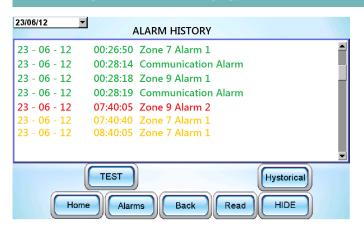
This page is available to collect all the loop's alarms. Inside this page is possible to see the type of Alarm, the Data and the time. There are three different colur:
