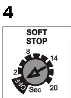
The **Soft Stop [off-20sec]** select the ramp time of Soft Stop. Stops gradually by delaying the time taken from the soft starter to bring the voltage to zero. The ramp time does not control the time required for the complete shutdown of the engine.
