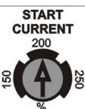
The **Start Current [150-250%]** select the initial current starting in % of Full Load Current.
