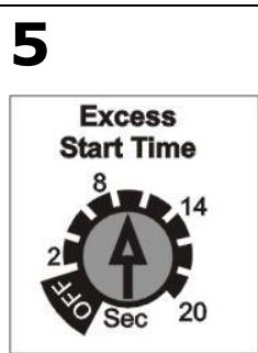
The **Excess Start Time [2-20sec]** configure protection against excessive starting time of the soft starter. Select a time slightly longer than that required by the engine for normal starting conditions. The soft starter will be in alarm mode if the start time is not completed within the selected time.
