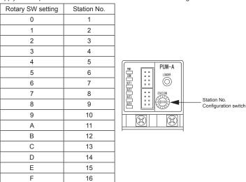
Each of connected controllers must have a different Station No. from other controllers. Duplicate Station No. may cause malfunction of the equipment.
