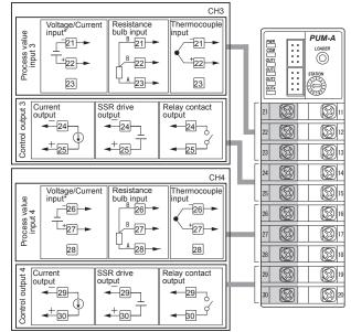
\*In case of currenet input, attach I/V unit which comes with the controller to the voltage input terminal.
