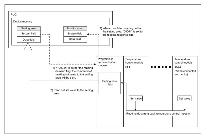
After reading out, execute the stop operation command 4-13 to put the programless communication module's reading demand into the standby status.
