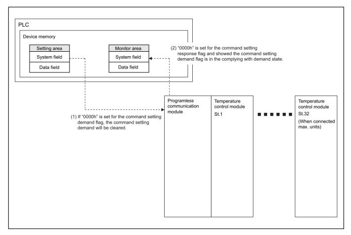
Executing this command puts the programless communication module into the standby status for the command setting demand.
