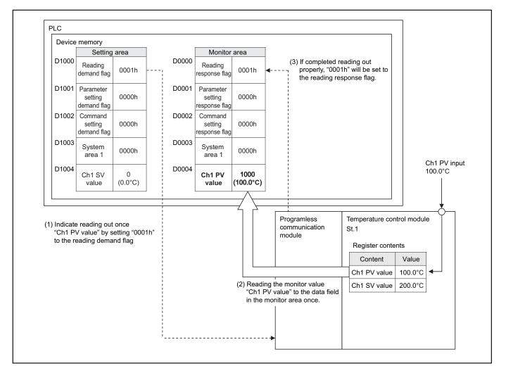
After reading out, set "0000h" (Stop operation)" to the reading demand flag (No. D1000) to put the programless communication module's reading demand into the standby status. When the reading demand comes to be in the standby, "0000h" will be set to the reading response flag (No. D0000).
