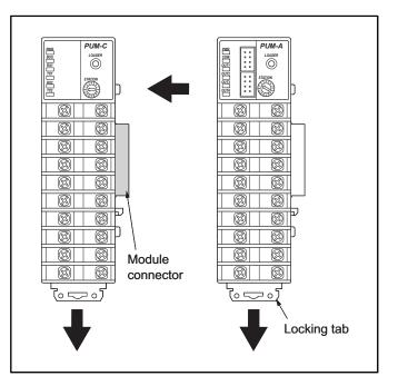
3. After mounting modules to the DIN rails, pull the all locking tabs up.
