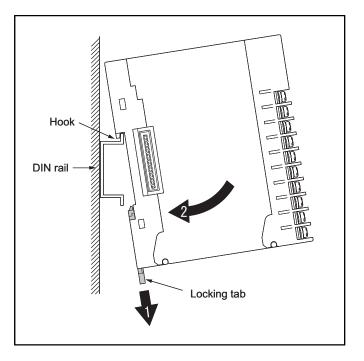
3. Pull up the locking tab of the base part to fasten the module onto the DIN rails.
