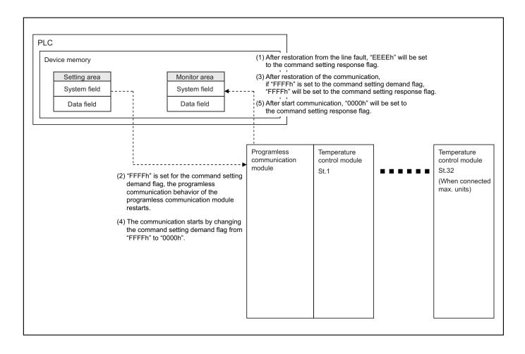
After communication restoration, execute the stop operation command module's command setting demand into the standby status.
