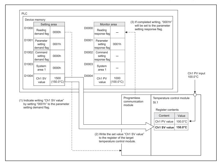
When "0001h" is set to the parameter setting demand flag (No. D1001), the value of the data field in the setting area (No.D1004) is written to "Control module (St. No. 1)'s Ch. 1 SV value", and "0001h" is set to the parameter setting response flag (No. D0001).
