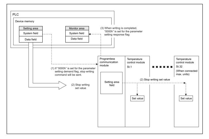
The programless communication module comes to be standby for the parameter setting demand with executing this command.
