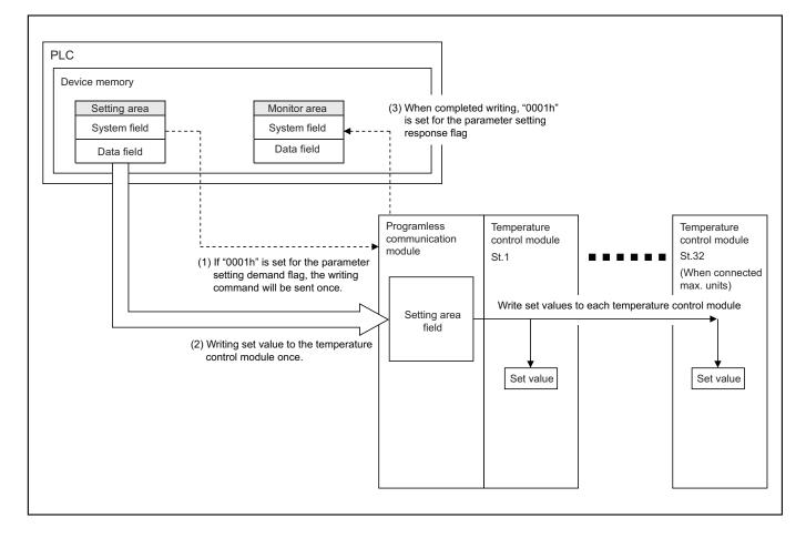
After writing, execute the stop operation command 4-18 to put the programless communication module's parameter setting demand into the standby status.
