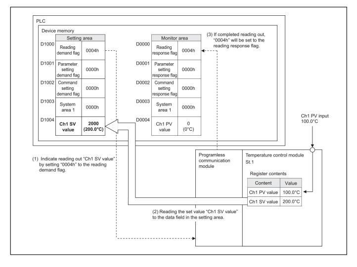
After reading out, set "0000h" (Stop operation) to the reading demand flag (No. D1000) to put the programless communication module's reading demand into the standby status. When the reading demand comes to be in the standby, "0000h" is set to the reading response flag (No. D0000).
