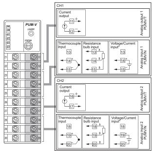
\*In case of currenet input, attach I/V unit which comes with the controller to the voltage input terminal
